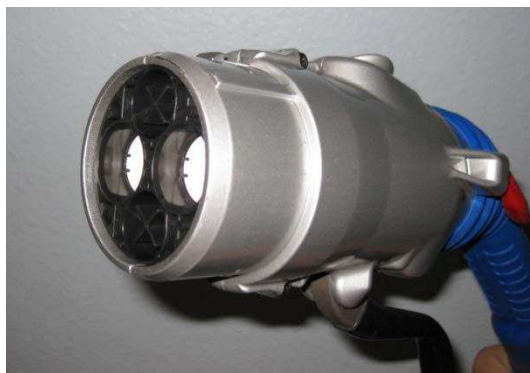
Figure 12. Direct current Level 2 charging CHAdeMO connector.
