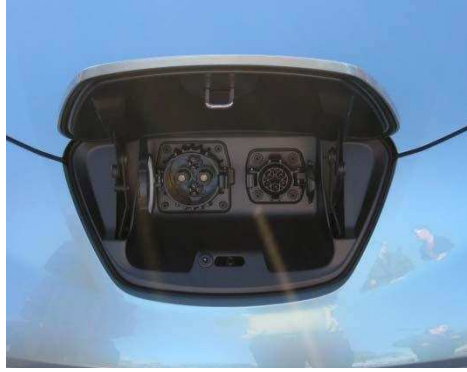
Figure 13. Nissan LEAF Level 2 inlets (direct current on left, alternating current on right).
