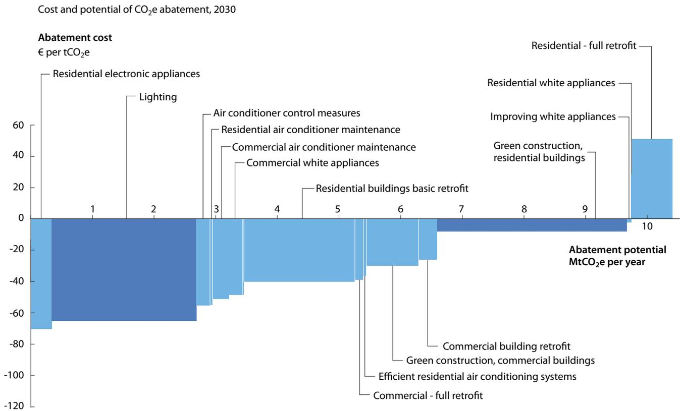
Note: The graph represents an estimation of the maximum GHG abatement potential of each of the technical levers at an economic cost below € 100/ton CO<sub>2</sub>e if all levers were to be fully implemented. It does not represent a prioritization of the various levers.
